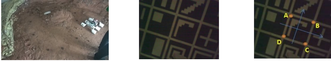
Figure 2 (a) The area of the mobile robot, (b) markers on the ceiling, (c) the photo with coordinates on the marker
