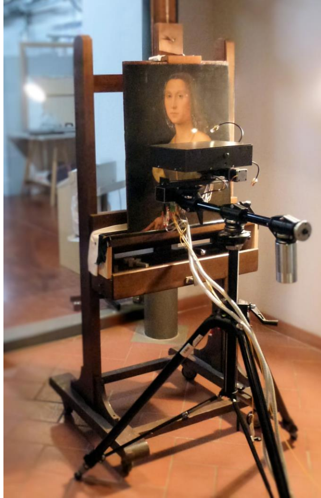
Figure 1. An in-situ examination of Raphael's La Muta in 2014 at Opificio delle Piere Dure in Florence, Italy with the portable OCT tomograph constructed at Nicolaus Copernicus University in Toruń
