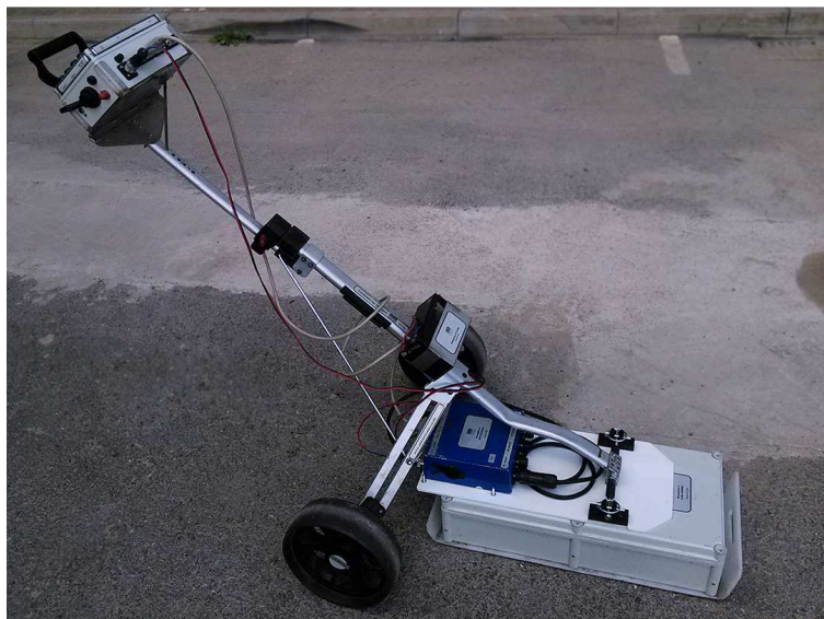
FIG. 5 – The GPR of the Crew 2 (400 MHz)
