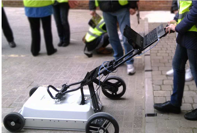
FIG. 4 – The GPR of the Crew 1 (250 MHz, 400 MHz and 1 GHz)
