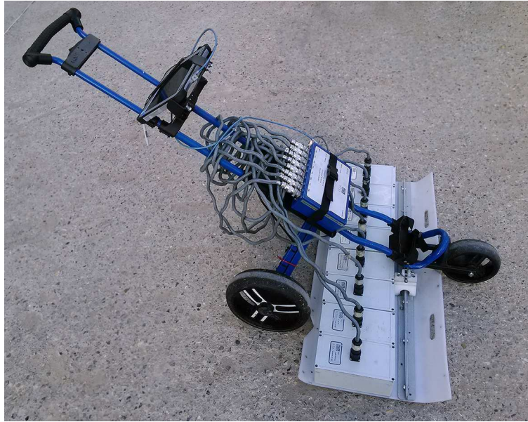
FIG. 6 – The GPR of the Crew 3 (8 channels)
