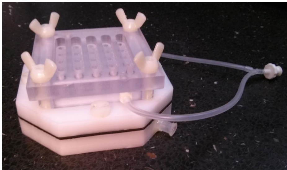
Fig. 1. An example of the fabricated parallel dot-blotter.
