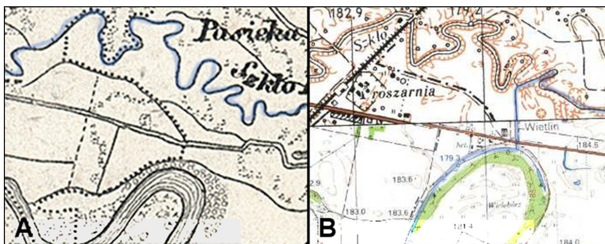
Fig. 7. Fragment of the 1855 Austrian map (A) and the 1980 raster map (B) showing the retained course of the river Szkło (old bed) and the canal leading to the San oxbow, currently the channel of the Motwica – stretches III and IV of the Motwica
