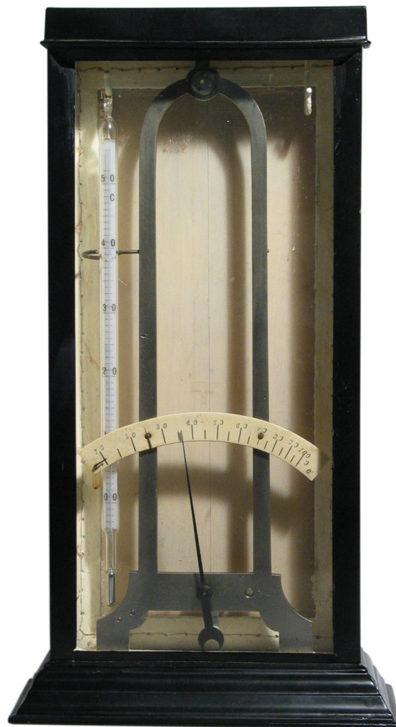
Fig. 2 Saussure-type hair hygrometer, manufactured by Hottinger & Cie, Zürich, ca. 1900. Image published with kind permission of the Technik Museum, Switzerland.
