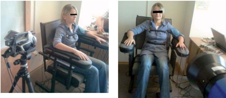
Fig. 2. Placement of thermal cameras during the experiment
