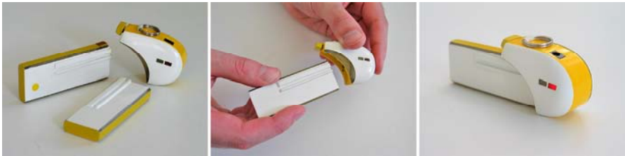
Fig. 6. Activation of the Personal.Aura artefact by connecting an ID Stick to the Reader Module
