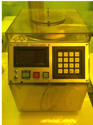
Figure 5.10: Spin coating apparatus located in Motlab, Tokyo University of Science.
