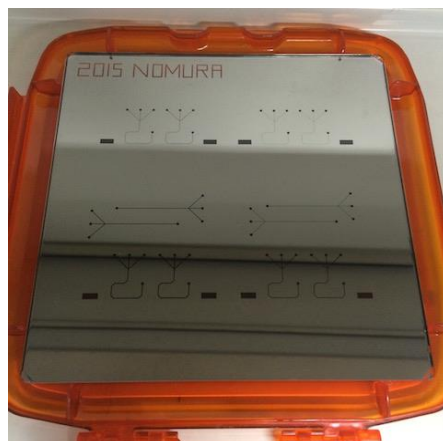
Figure 5.6: Photomask used in the microfluidic channel development, created by Sayaka Nomura in 2015.
