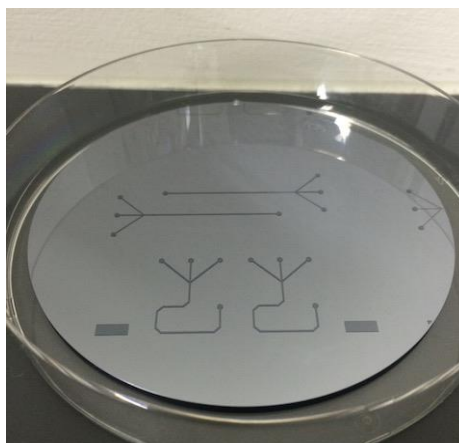
Figure 5.12: Silicon wafer microfluidic channel master mould.
