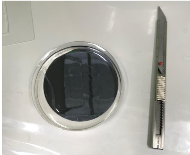
Figure 5.14: Final microfluidic PDMS channel before assembly.
