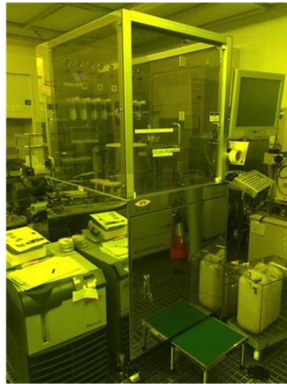
Figure 5.4: Automatic photomask developing system. Located in Tokyo University.
