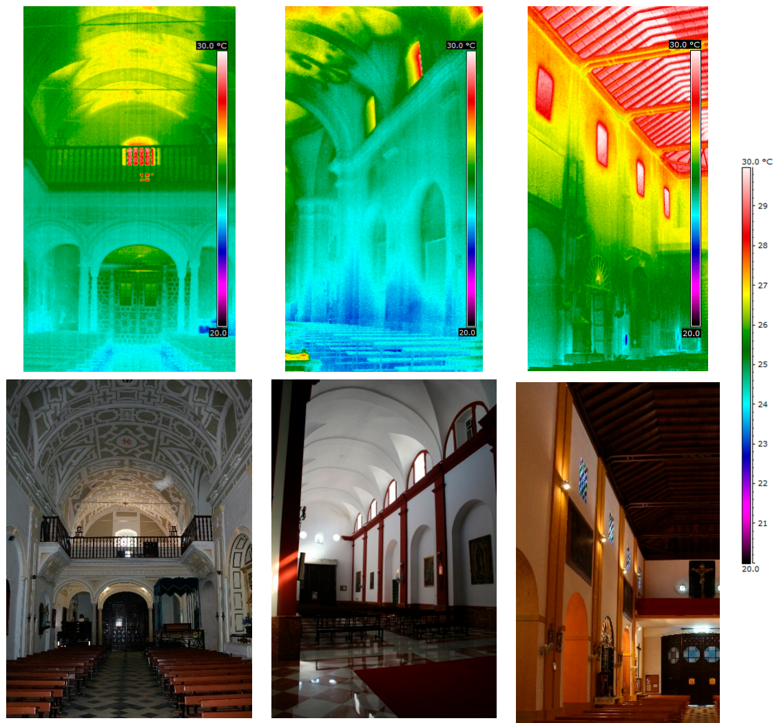
Figure 2. Surface Temperatures in June. (SF) San Francisco de Asís Church, (M) Nuestra Señora de la Merced Church, and (V) Nuestra Señora de la Victoria Church.
