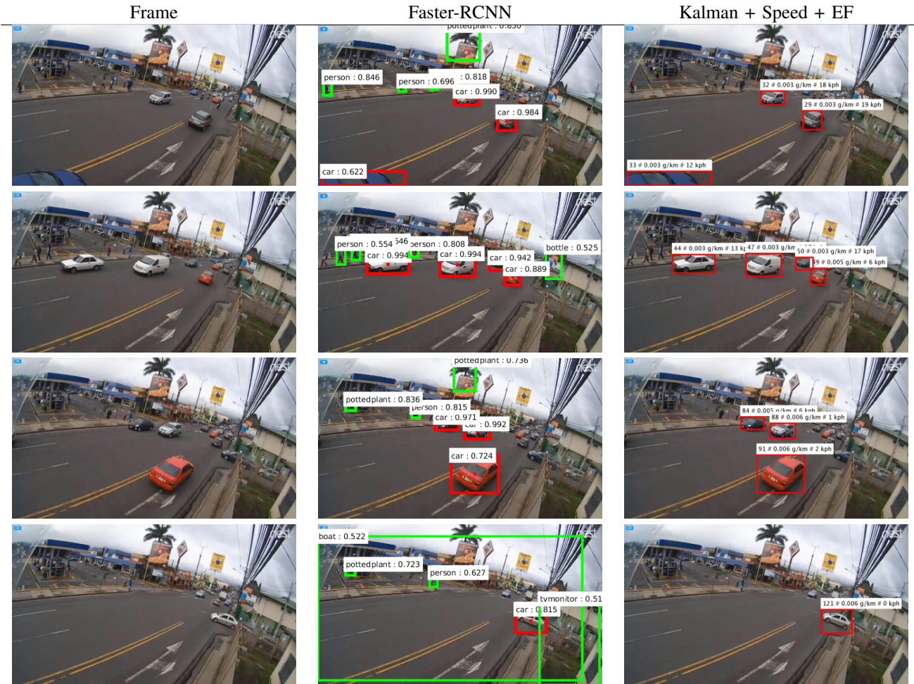
Figure 5. Graphical description of the operation of the proposed method. From left to right, the columns show a frame of a sequence, the objects detected on it provided by the Faster-RCNN module, and the detected cars with the trajectory given by the Kalman model, and speed and pollution estimation information. The rows show frames 698, 1000, 1651 and 2563 of camara-guadalupe . Note that the red bounding boxes correspond to undesired object detected and the green bounding boxes correspond to the objects which belong to the car class.
