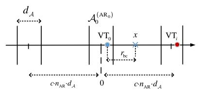
Figure 7.3: Illustration of co-channel segments in the abstraction model. The probe transmitter is represented as VT<sub>0</sub>, the probe AR and segment as AR<sub>0</sub> and  $\mathcal{A}_0^{(AR_0)}$  respectively, the probe receiver as a blue x and a single interfering vehicle as VT<sub>i</sub>. The length of each segment is represented as  $d_A$  and thus  $n_{AR} \cdot d_A$  is the minimum co-channel distance.
