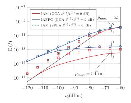
Figure 3.3: Mean of the interference versus  $i_0$  for IAM and IAFPC methods with  $\epsilon = 1$ ,  $p_{\text{max}} \rightarrow \infty$  and  $p_{\text{max}} = 5$  dBm.
