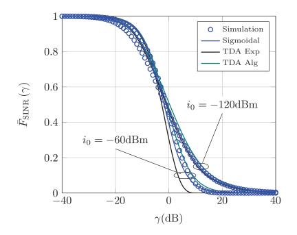
Figure 2.6: ccdf of the SINR for the typical MT (IAFPC is assumed) with  $\epsilon = 1$  and  $i_0 = \{-120, -60\}$  dBm.
