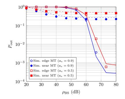
Figure 6.3: Comparison of the outage probability for near and cell-edge MTs versus the transmit SNR,  $\rho_{\rm BS}$ . The case  $a_e = 0.9$  is represented with blue color and circles and the case  $a_n = 0.5$  with red color and squares.
