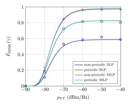
Figure 7.13: Capture probability versus the transmit power per Hz,  $\rho_{\rm VT}$ , for SLP ( $d_{\rm safe} = 0$  m) and for MLP ( $d_{\rm safe} = 42$  m) with periodic and non-periodic broadcast messages.
