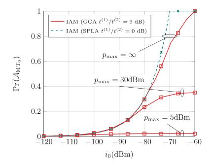
Figure 3.2: Probability of being active of the typical MT for IAM with  $\epsilon = 1$ ,  $p_{\text{max}} \to \infty$ ,  $p_{\text{max}} = 30$  dBm and  $p_{\text{max}} = 5$  dBm.
