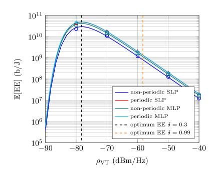
Figure 7.14: Average EE versus the transmit power per Hz,  $\rho_{\rm VT}$ , for SLP ( $d_{\rm safe} = 0$  m) and for MLP ( $d_{\rm safe} = 42$  m) with periodic and non-periodic broadcast messages.
