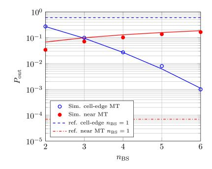
Figure 6.4: Comparison of the outage probability for near and cell-edge MTs versus the number of BSs per cluster,  $n_{\rm BS}$  for  $a_e = 0.9$ . The special case  $n_{\rm BS} = 1$  is added as a reference value for comparison.
