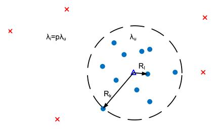
Figure 4.2: Multi-User UL set-up based on conditional thinning for k = 11. Interfering users for the  $l^{th}$  user transmission are represented with red crosses.
