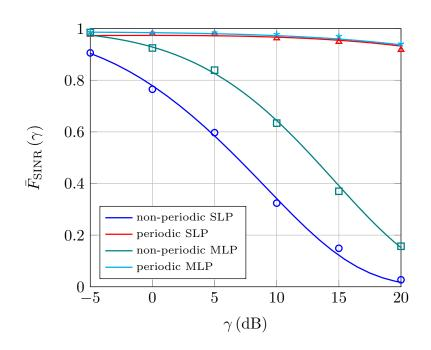
Figure 7.4: Capture probability versus the SINR threshold,  $\gamma$ , for SLP ( $d_{\text{safe}} = 0$  m) and for MLP ( $d_{\text{safe}} = 42$ ) with periodic and non-periodic broadcast messages. Analytical results are represented with solid lines whereas simulation results are represented with marks.
