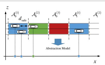
Figure 7.1: Sketch of GLOC based access with SLP for a two-lane road and 3 ARs. Different colors are associated to different ARs. On the bottom it is shown the abstraction model for the study of the road where positions of vehicles are treated as points in the real line.
