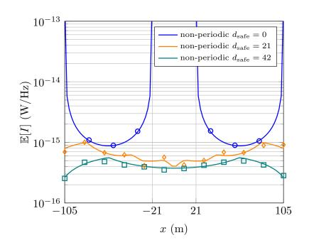
Figure 7.10: Average interference for different locations,  $x \in [-105, +105]$  m, for SLP and MLP with  $d_{\text{safe}} = \{21, 42\}$  with non-periodic messages,  $\lambda = 0.8/84$  vehicles/m and  $n_{\text{AR}} = 3$ .
