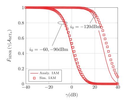
Figure 3.6: CCDF of the SINR for the typical MT conditioned on being active for IAM with  $\epsilon = 0.75$ ,  $t^{(1)}/t^{(2)} = 9$  dB,  $p_{\text{max}} \to \infty$  and  $i_0 = \{-120, -90, -60\}$  dBm.
