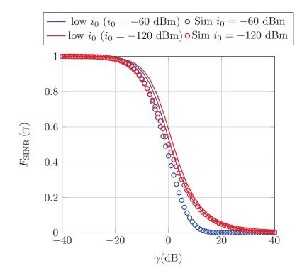
Figure 2.7: ccdf of the SINR in the low  $i_0$  regime given by (2.46) and by using the minimum path loss association.
