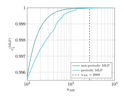
Figure 7.8: Maximal capture probability,  $c_1^{(\text{MLP})}$ , for  $n_{\text{AR}}$  ranging from  $10^2$  to  $10^4$ , under MLP ( $d_{\text{safe}} = 42 \text{ m}$ ) with periodic and non-periodic broadcast messages with  $r_{\text{bc}} = 150 \text{ m}$ ,  $d_{\text{max}} = 56 \text{ km}$  and  $\gamma = 5 \text{ dB}$ .
