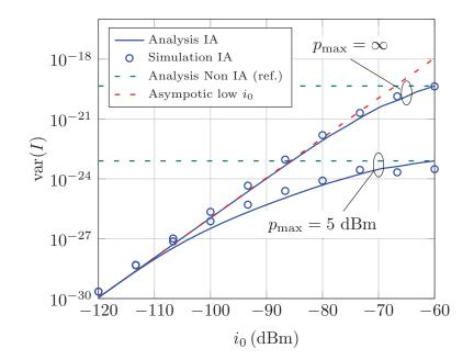
Figure 2.4: Variance of the interference versus  $i_0$  for IAFPC and non-IA FPC with  $\epsilon = 1$ ,  $p_{\text{max}} \rightarrow \infty$  and  $p_{\text{max}} = 5$  dBm.
