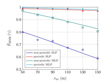
Figure 7.11: Capture probability versus the broadcast distance,  $r_{\rm bc}$ , for SLP ( $d_{\rm safe} = 0$  m) and for MLP ( $d_{\rm safe} = 42$  m) with periodic and non-periodic broadcast messages.
