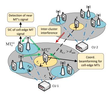
Figure 6.1: Illustration of the proposed NOMA-based scheme with coordinated beamforming for CRANs. The probe near MT and probe cell-edge MT are represented as  $MT_0^{(n)}$ and  $MT_0^{(e)}$ , respectively. It is drawn a single interfering cluster, which is centered at x.
