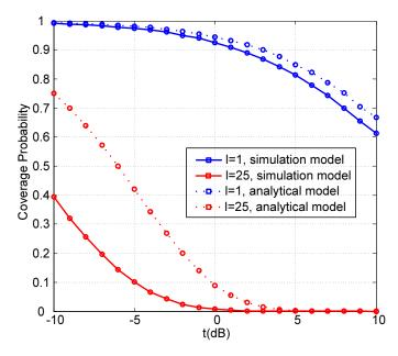
Figure 4.7: Coverage probability for cell-interior l = 1 and cell-edge l = k with k = 25, without power control  $\epsilon = 0$ , without noise,  $\alpha = 2.5$ ,  $\lambda_b = 0.24$
