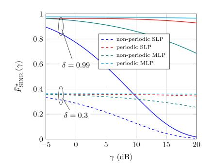
Figure 7.16: Capture probability versus the SINR threshold,  $\gamma$ , associated with the optimum transmit power,  $\rho_{\rm VT}^{\star}$  as appear in Fig 7.15.
