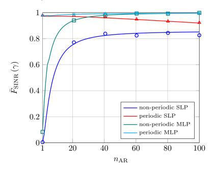
Figure 7.7: Capture probability versus the number of ARs,  $n_{\text{AR}}$ , for SLP ( $d_{\text{safe}} = 0 \text{ m}$ ) and for MLP ( $d_{\text{safe}} = 42 \text{ m}$ ) with periodic and non-periodic broadcast messages.
