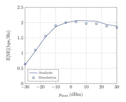
Figure 2.9: Average SE versus  $p_{\text{max}}$  (IAFPC is assumed) for  $i_0 = -90$  dBm.
