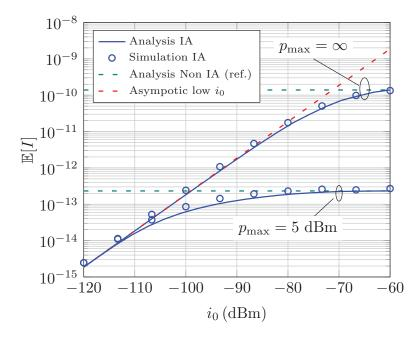
Figure 2.3: Mean of the interference versus  $i_0$  for IAFPC and non-IA FPC with  $\epsilon = 1$ ,  $p_{\text{max}} \rightarrow \infty$  and  $p_{\text{max}} = 5$  dBm.
