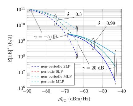
Figure 7.15: Optimum EE versus the optimum transmit power per Hz,  $\rho_{\rm VT}^{\star}$ , for SLP  $(d_{\rm safe} = 0 \text{ m})$  and for MLP  $(d_{\rm safe} = 42 \text{ m})$  with periodic and non-periodic broadcast messages. Each pair of values ( $\mathbb{E}[\text{EE}]^{\star}, \rho_{\rm VT}^{\star}$ ) is obtained for a different SINR threshold,  $\gamma$ , ranging from -5 dB to 20 dB.
