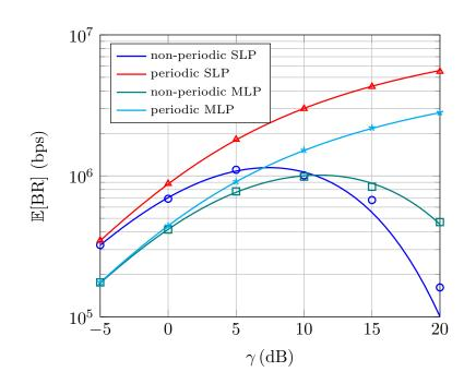
Figure 7.5: Average BR versus the SINR threshold,  $\gamma$ , for SLP ( $d_{\text{safe}} = 0 \text{ m}$ ) and for MLP ( $d_{\text{safe}} = 42 \text{ m}$ ) with periodic and non-periodic broadcast messages.
