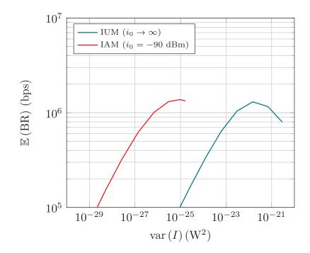
Figure 3.10: Average BR as a function of the variance of the interference for IAM ( $i_0 = -90$  dBm) and IUM ( $i_0 \rightarrow \infty$ ) schemes with  $p_{\text{max}} = 5$  dBm and  $t^{(1)}/t^{(2)} = 9$  dB.
