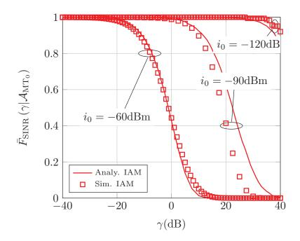
Figure 3.5: CCDF of the SINR for the typical MT conditioned on being active for IAM with  $\epsilon = 1$ ,  $t^{(1)}/t^{(2)} = 9$  dB,  $p_{\text{max}} \to \infty$  and  $i_0 = \{-120, -90, -60\}$  dBm.
