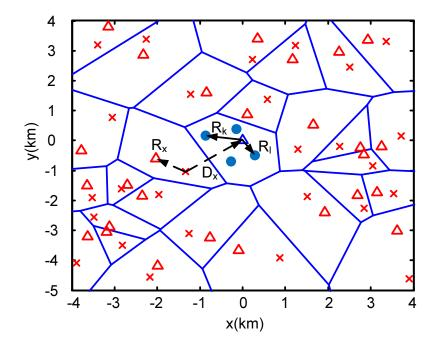
Figure 4.1: System model of multi-user UL cellular system. BSs are represented by triangles (blue: serving BS), scheduled users inside the serving cell are represented by blue dots, interfering users for the  $l^{th}$  user transmission are depicted with a red cross. The distance from one interfering user to its serving BS  $(R_x)$  and to the target BS  $(D_x)$  are represented as an example. Only scheduled users are represented.
