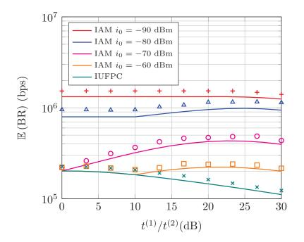
Figure 3.12: Average BR as a function of  $t^{(1)}/t^{(2)}$  for IUFPC  $(i_0 \to \infty)$  and IAM with  $i_0 = \{-90, -80, -70, -60\}$  dBm.  $p_{\text{max}} \to \infty$  for both schemes.
