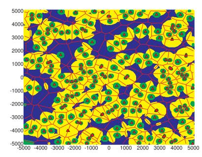
Figure 2.1: Homogeneous network realization in  $[-5000, 5000]^2$  m<sup>2</sup> showing with green color the positions related to non truncated MTs. Yellow and blue colors are associated with MTs truncated by  $i_0$  and to  $p_{\text{max}}$ , respectively. The simulation parameters are  $\lambda^{(1)} = 2$ BS/km<sup>2</sup>,  $i_0 = -90$  dBm,  $p_{\text{max}} = 30$  dBm,  $p_0 = -70$  dBm and  $\epsilon = 1$ .
