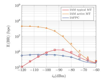
Figure 3.8: Comparison of average BR of IAFPC and IAM for  $\epsilon = 1$ ,  $t^{(1)}/t^{(2)} = 9$  dB and  $p_{\text{max}} \to \infty$ . As for IAM, two cases are considered: the typical MT and the typical active MT.
