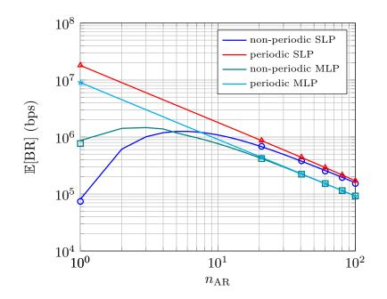
Figure 7.9: Average BR versus the number of ARs,  $n_{\text{AR}}$ , for SLP ( $d_{\text{safe}} = 0$  m) and for MLP ( $d_{\text{safe}} = 42$  m) with periodic and non-periodic broadcast messages.
