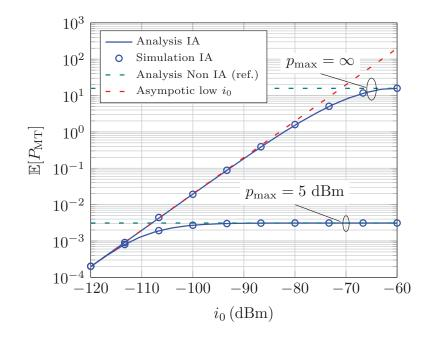
Figure 2.2: Average transmitted power versus  $i_0$  for IAFPC and non-IA FPC with  $\epsilon = 1$ ,  $p_{\text{max}} \rightarrow \infty$  and  $p_{\text{max}} = 5$  dBm.
