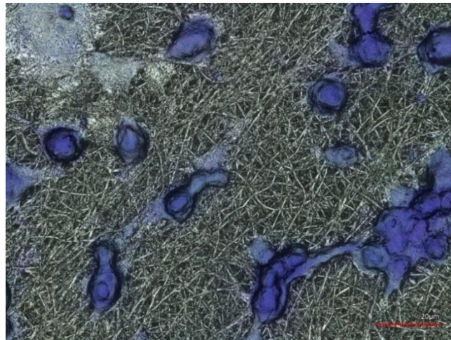
Fig. 1.6 CLSM images of CHO-DP12 (Chinese hamster ovary strain DP12) cells, colored with methylene blue on a PAN/gelatin blend nanofiber mat. The scale bar indicates 20 μm.
