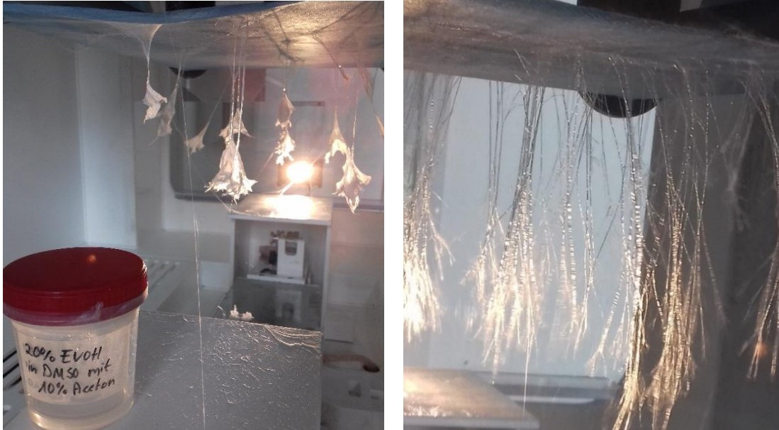
Fig. 1.3 Examples of different artefacts occurring by needleless electrospinning process during this PhD project.
