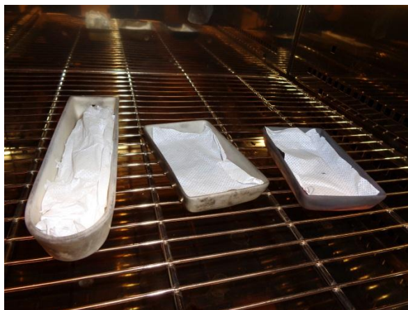
Fig. 6.1 Multi-layer nanofiber mat (left boat) and single-layer nanofiber mats (middle and right boat) in the stabilizing oven.
