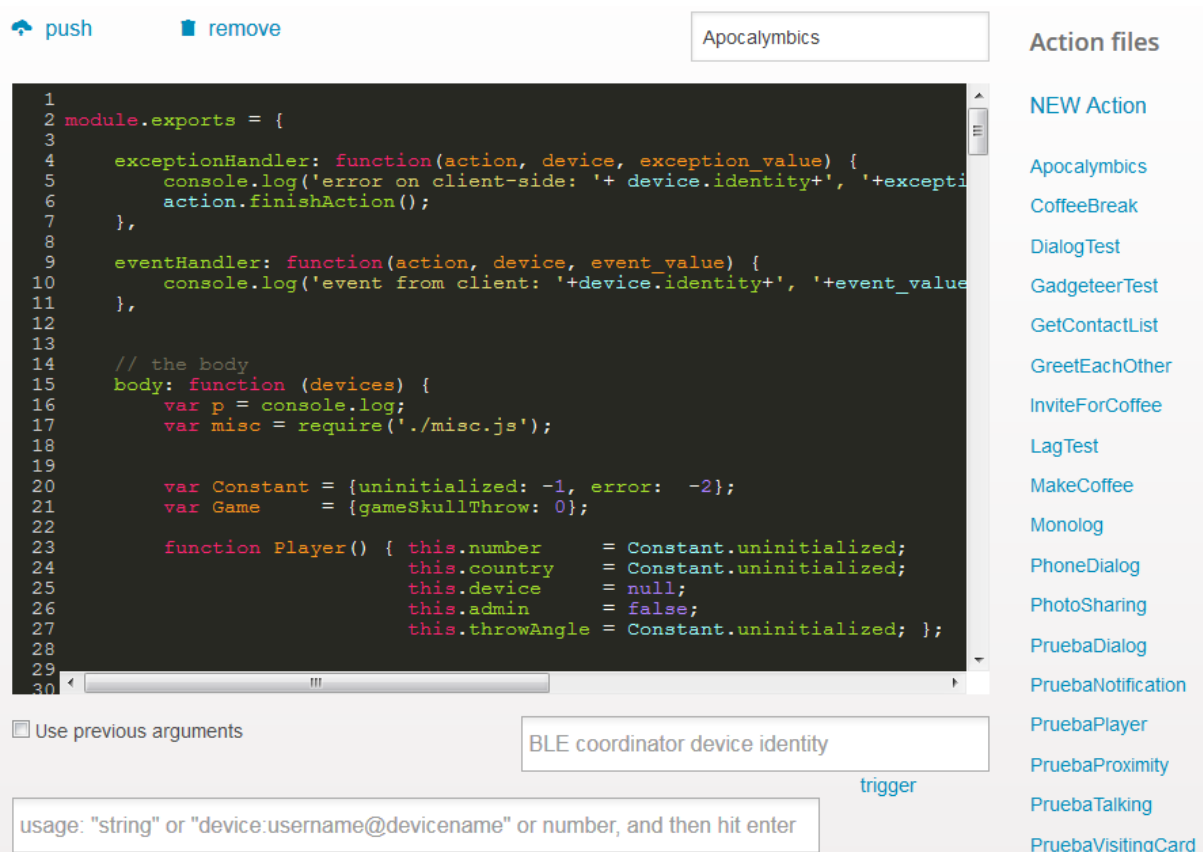
Figure 15. Example of the Actions Definition view, with the Apocalymbics action loaded in the editor.
