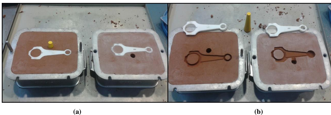
Figure 1: Sand casting process. Open mold with patterns and sprue inserted (a) and mold with pattern extracted ready to be closed (b)
