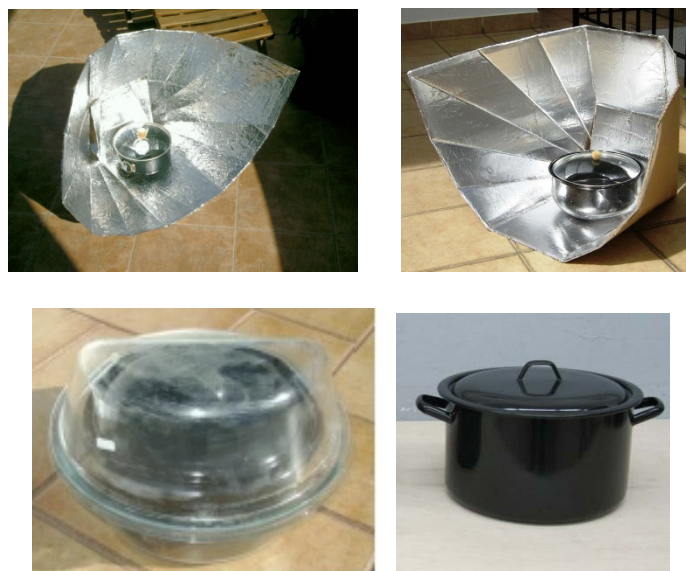
Figure 1. Pictures of a solar funnel cooker by Teong Tan [10] (top), of a transparent enclosure (bottom left) and a black cooking vessel (bottom right).
