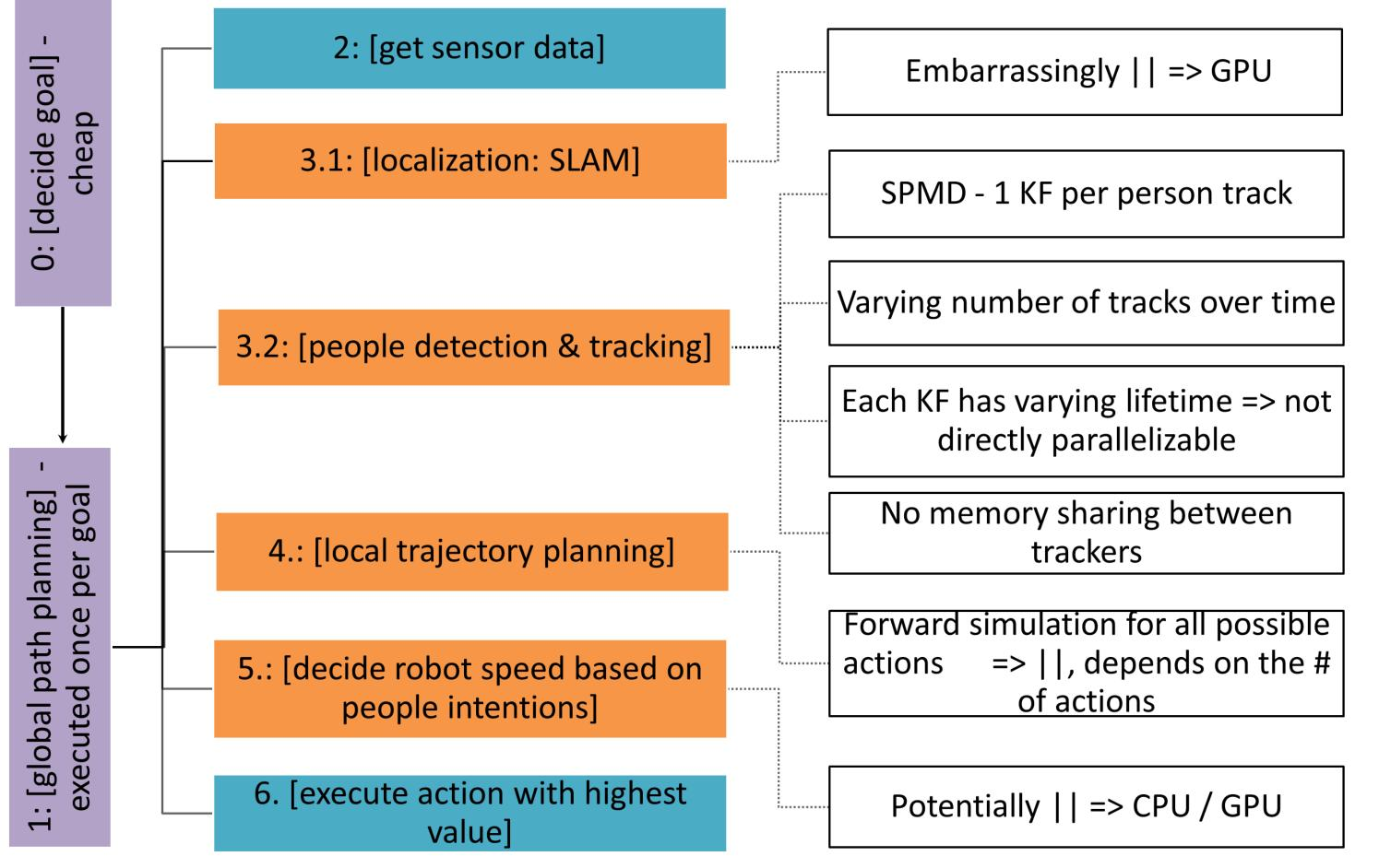
Next steps - meet low-power & real-time requirements using parallelized implementation on low-power high-performance accelerator hardware
