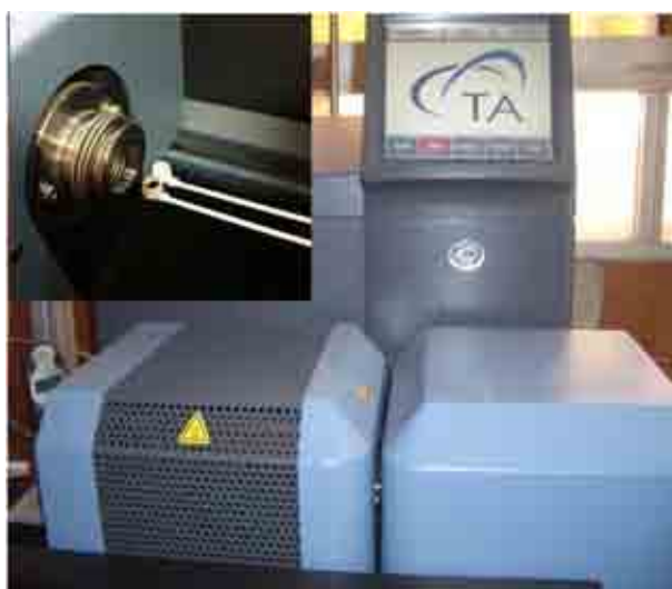
Figure 2.2. SDT Q600 Thermobalance with the detail of the sample pans.
