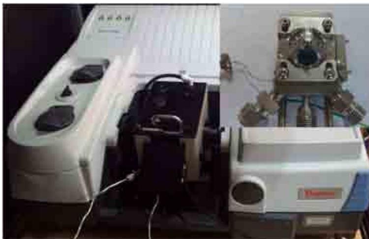
Figure 2.1. Nicolet Nexus 6700 Spectrometer with the DRIFT reaction chamber, which is shown in the inset.
