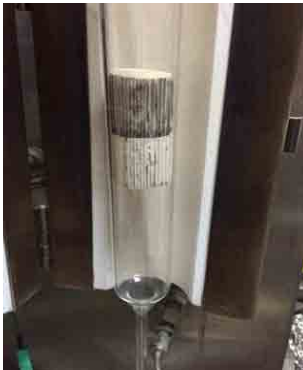
Figure 5.16. Double bed configuration system for experiments with monoliths.
