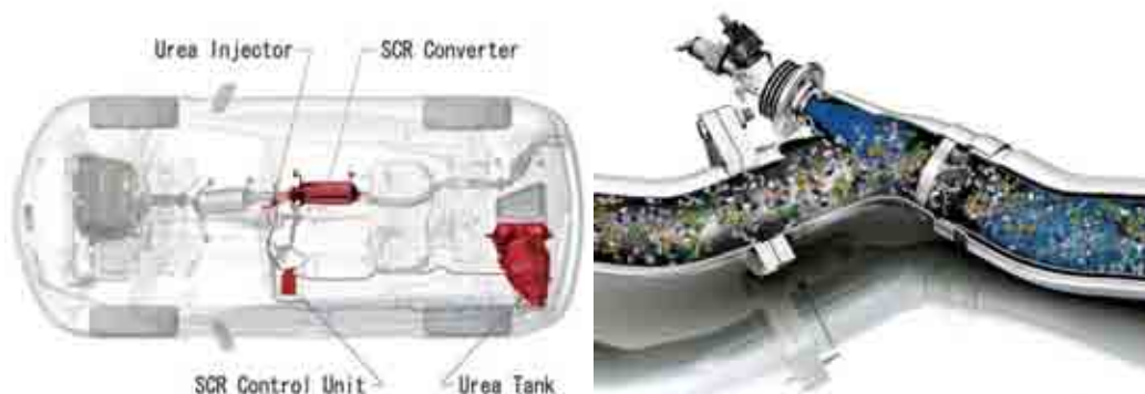
Figure 1.4. Vehicle diagram of the Urea system and the detail of the mixture.
