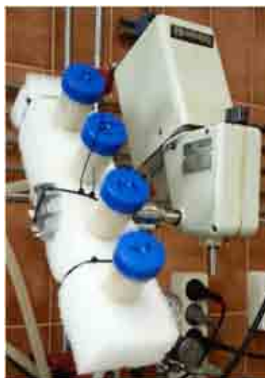
Figure 2.4. Rotation system for the synthesis of monoliths.
