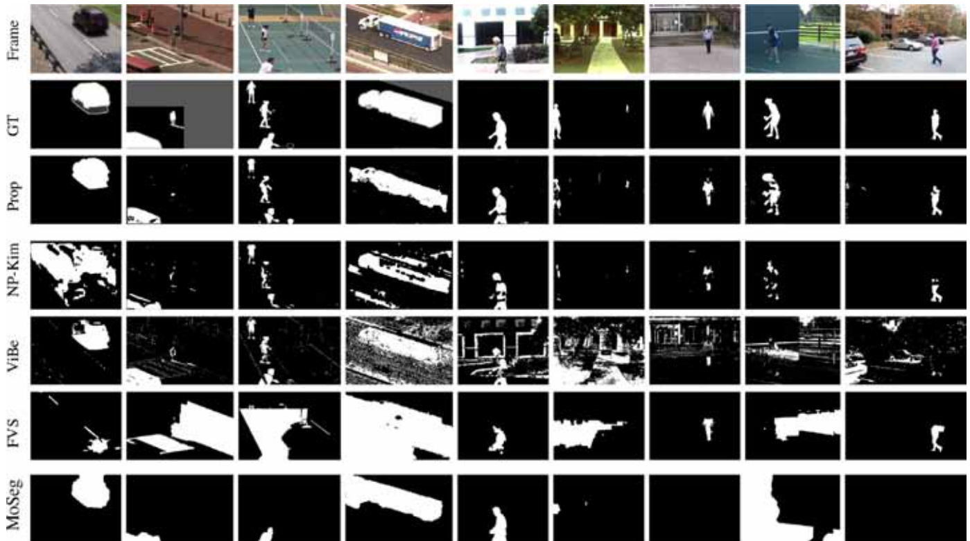
Fig. 4. Results for the sequences using the best configuration according to F-measure. From left to right: traffic, sidewalk, badminton, boulevard, campus1, campus2, campus3, tennis and woman. Rows from up to down: original frame, ground truth frame, proposed method, NP-Kim, ViBe, FVS and MoSeg.
