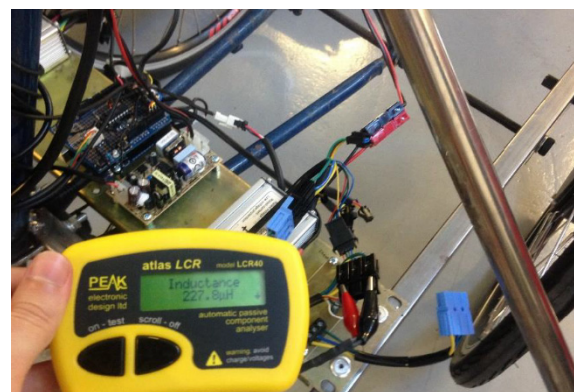
Fig. 3 Initial characterization of the engines of the tricycle.
