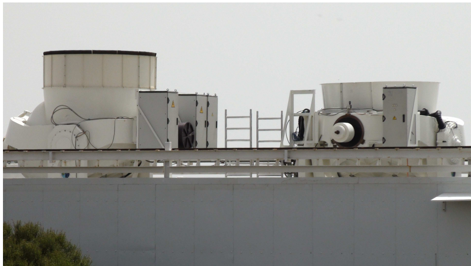
FIGURE 3.5— Photograph of the QT1 and QT2. QT1 on the left is equipped with the extended shield that avoids the spillover which causes far sidelobes from the strong astronomical sources, especially the geostationary satellites. On the contrary, the QT2 is not expected to be affected since it observes at higher frequency (30 and 40 GHz), where no geostationary satellites emission is expected. QT1 was an exact replica of QT2 before April 2014, when the shield was installed.
