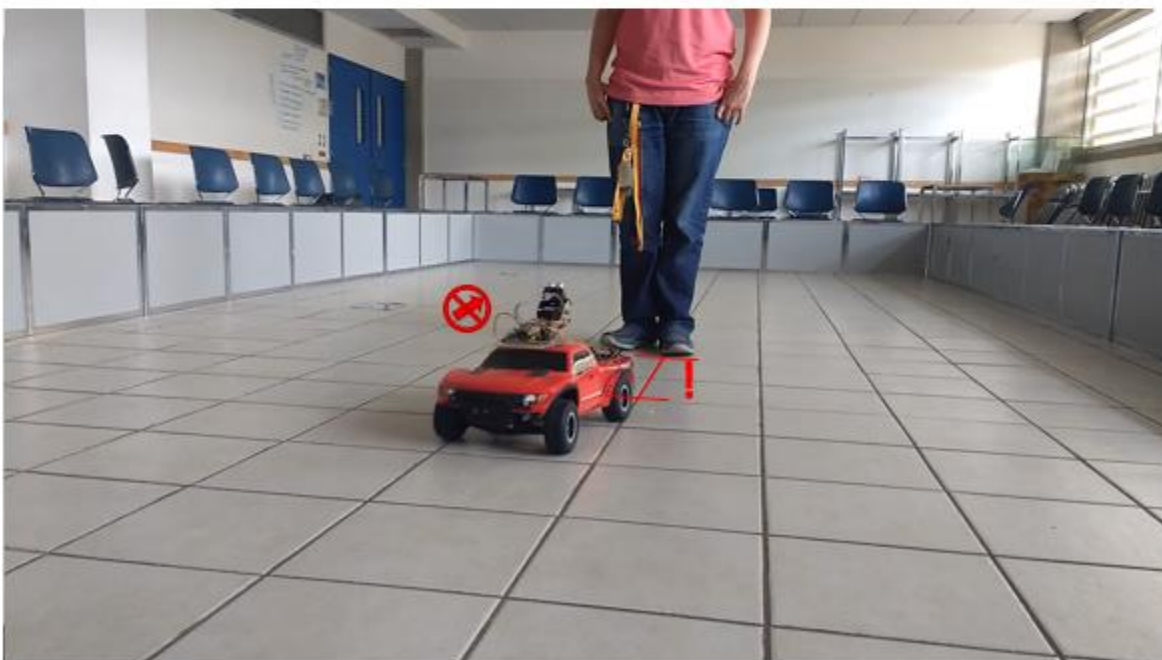
b) The person stops. When the distance threshold is reached, the vehicle ceases its movement.
