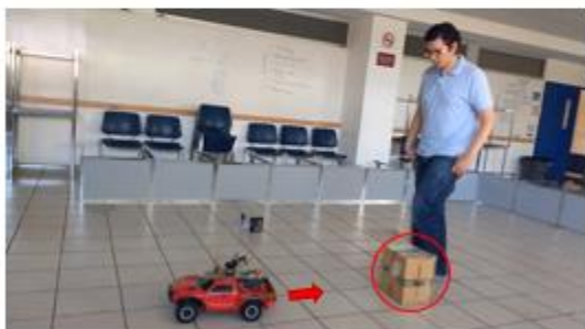
b) The person passes over the obstacle. The vehicle continues its movement towards the user.
