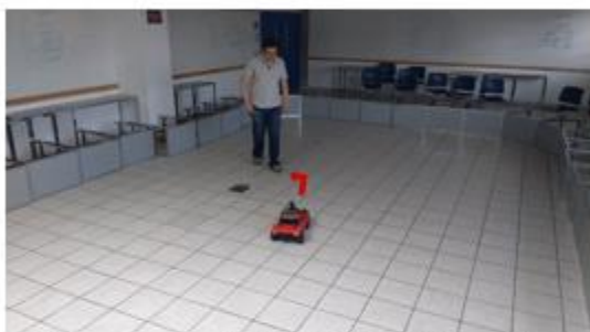
b) Person moves to the left, the vehicle starts steering accordingly in order to follow the person.
