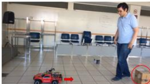
a) The vehicle starts to follow the person. A far away obstacle is present on the vehicle's path.
