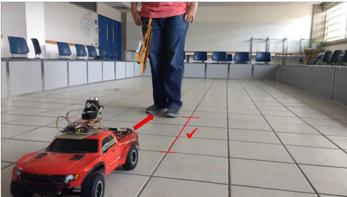
a) The vehicle accelerates after detecting a person's face, and determining that the person is far away.
