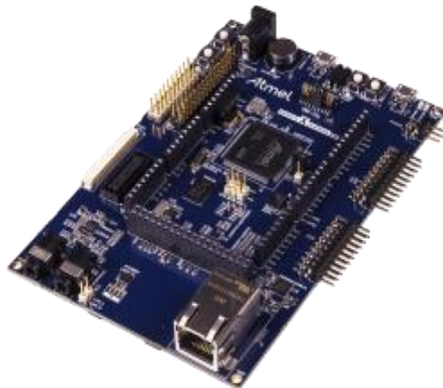
Figure 2-10: SAM V71 Ultra Evaluation Kit PCB [24].
