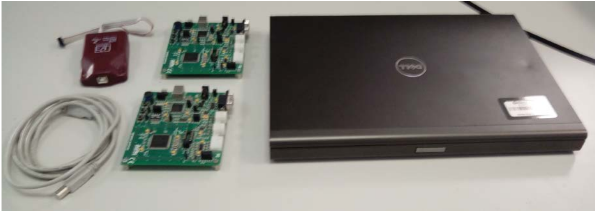
Figure 4: Used set up of LIN protocol communication tests: a Laptop, two DEMO9S12XEP100 boards, a P&E USB-Multilink-Interface debugger and a USB to Serial adapter.
