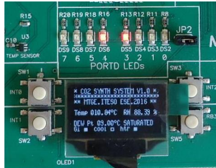
Figure 23. System captured 5 mins later: Temp increasing and RH% decreasing
