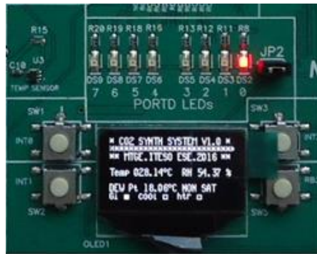
Figure 24. System at 30 mins later: Room temp reached, nominal RH% reached, DESAT OFF
