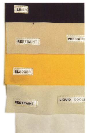
ILC Dover, manufacturer, eleven layers of material for Extravehicular Mobility Unit (textile sample), ca. 1983. Gift of ILC Industries, Inc./ ILC Dover
