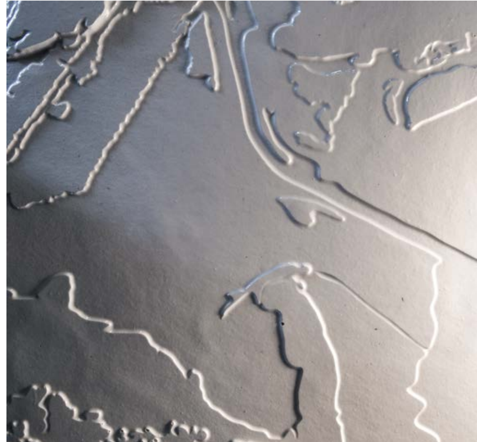
A regional splash model was cast out of a vacuum-formed polystyrene mold.
