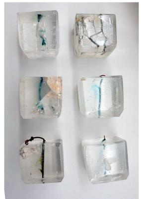
Assorted inclusion specimens: wire, clay, plaster, plaster + silica, fibre glass tape, etc.
