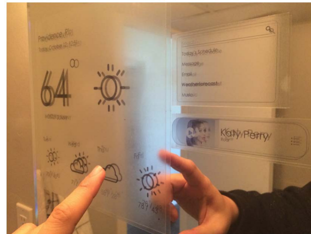
Figure 16: Weatherforecast GUI on the bathroom glass and near the lighting switch. To explore specifically, I chose several surfaces which are suitable for attaching it as a venue for getting provided weather information: The left picture on the top is when I attached a sticker right beside a lighting switch on the wall of the living room. The rest of the pictures show that I attached it to the mirror in the bathroom. To explain this situation, I thought about general behavioral patterns that most people show in a process of perceiving daily information or interplaying with applications through smart devices (e.g., weather information, schedule, playing music they like, etc.) in morning.
