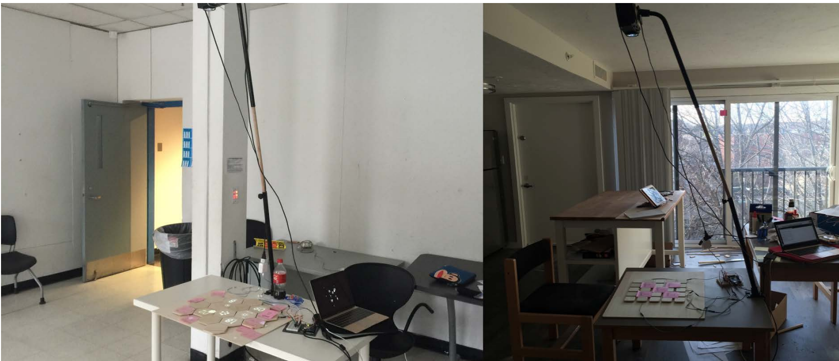
Figure 81 - 1: To perpendicularly project the GUIs onto a surface, I attached a small sized projector to a frame I modified.
