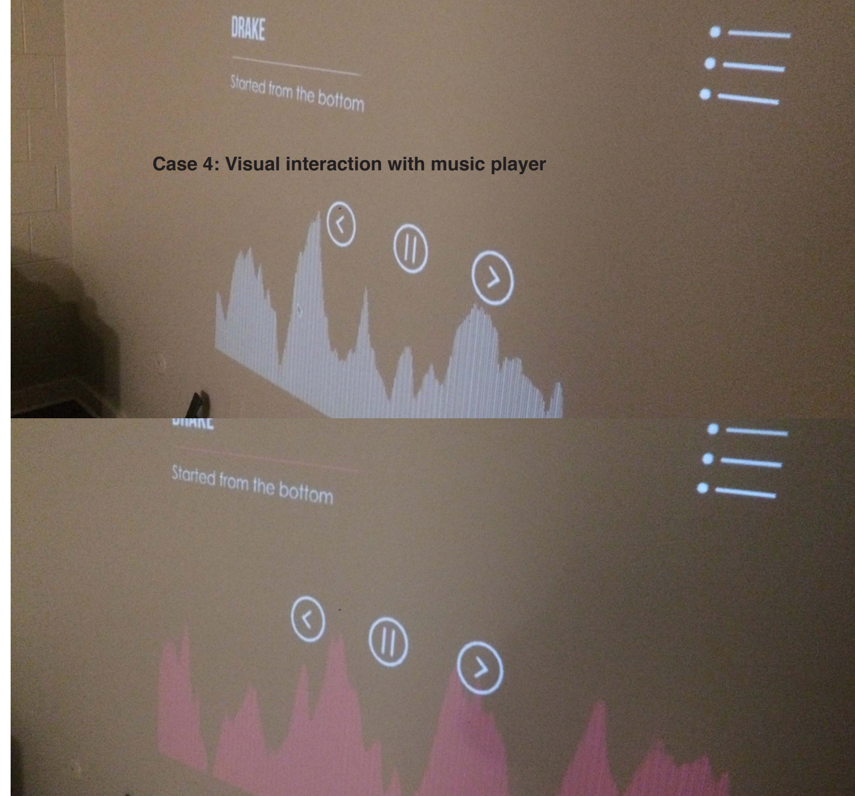
Figure 61: The color of sound wave changes into different colors in correspondence with the next song's tone.
