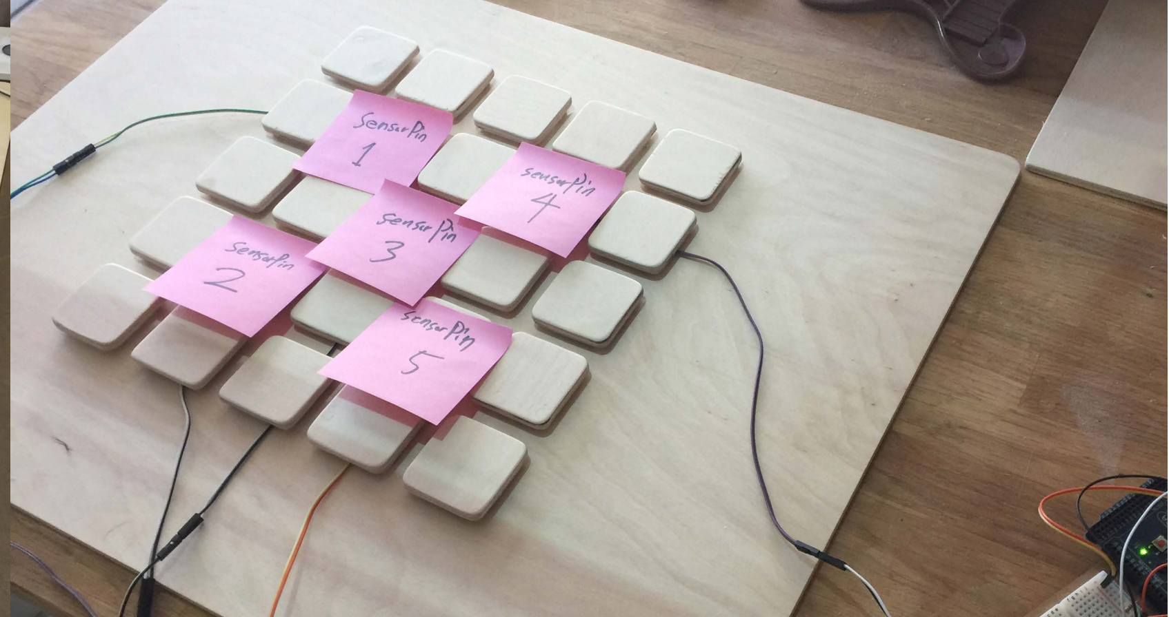
Figure 81 - 6: This is the moment of simultaneously re-adjusting the coordinate of GUIs while projecting it on a surface. To easily synchronize the graphic interaction with physical grids, I marked the sensor's position as above by using post-it notes.
