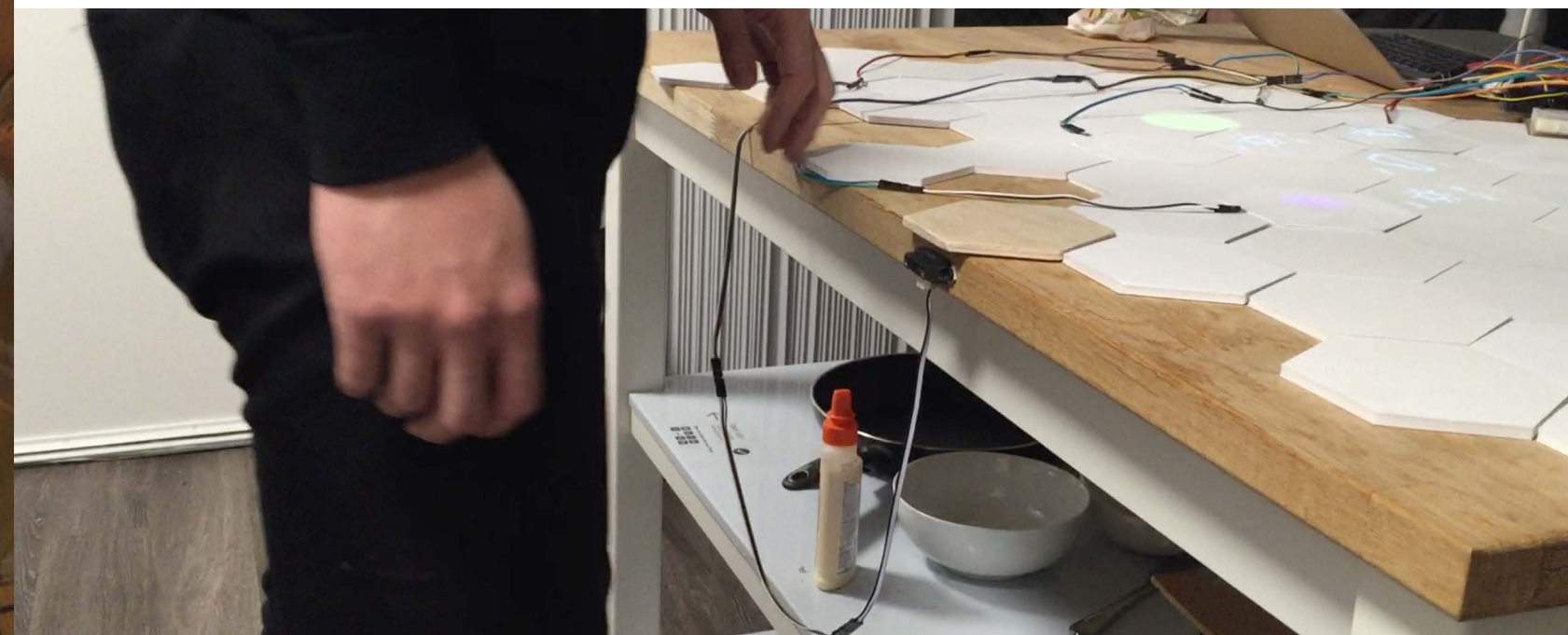
Figure 89: Based on the idea that interaction is activated by user's approach, I attempted to set up the IR sensor under the surface to read user's reach. Different to Figure 95's thermo sensor, IR sensor's value flow was relatively stable, but the sensor frequently generated irregular, uncontrollable interactions. Because of that, it is still required to being eased down especially when people get close to it.
