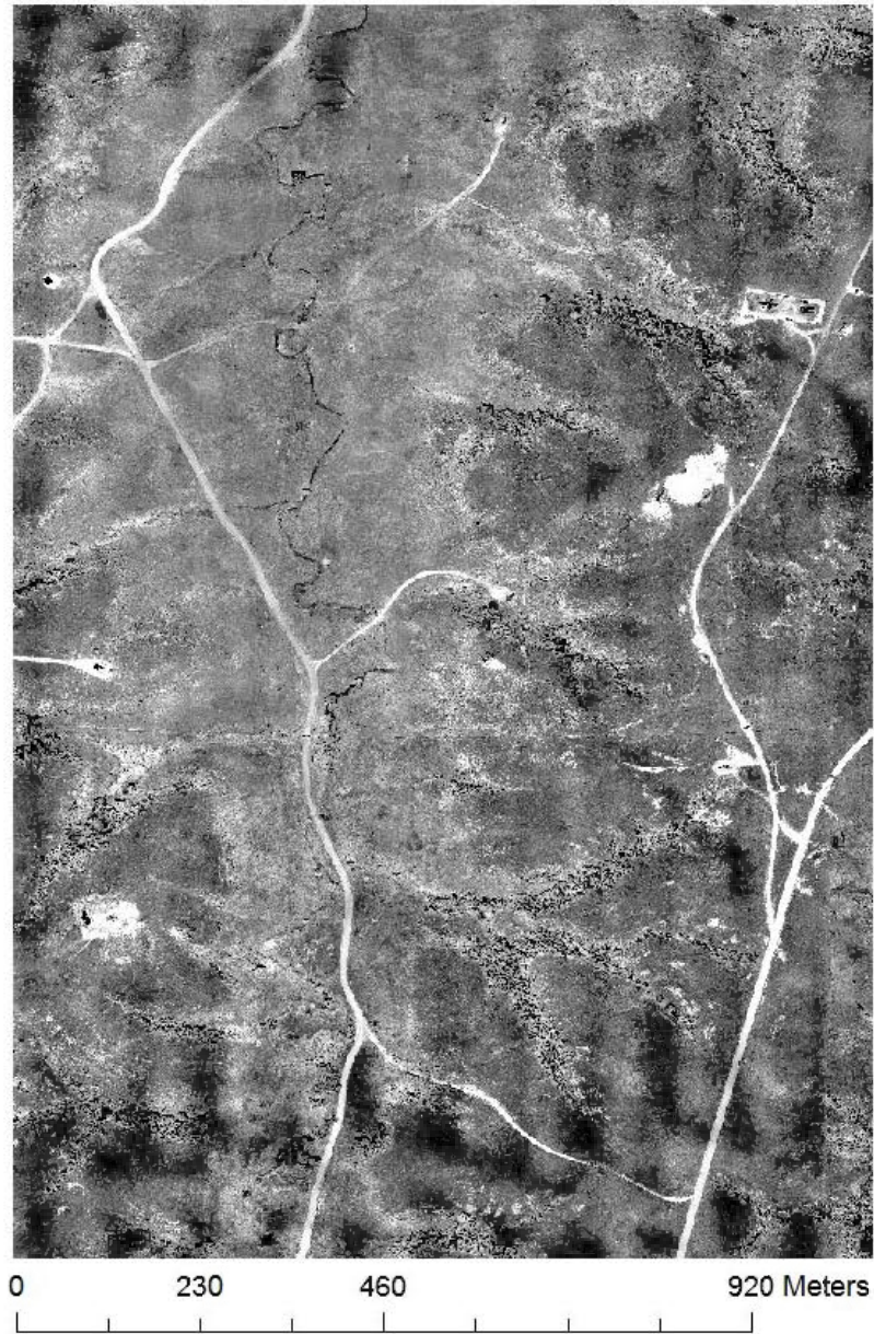
Figure 18: Orthomosaic of the Training plot generated in Agisoft Photoscan at Hadley Ranch and the Near-infrared light (~710 nm) reflectance values. Images were captured in July, 2017.
