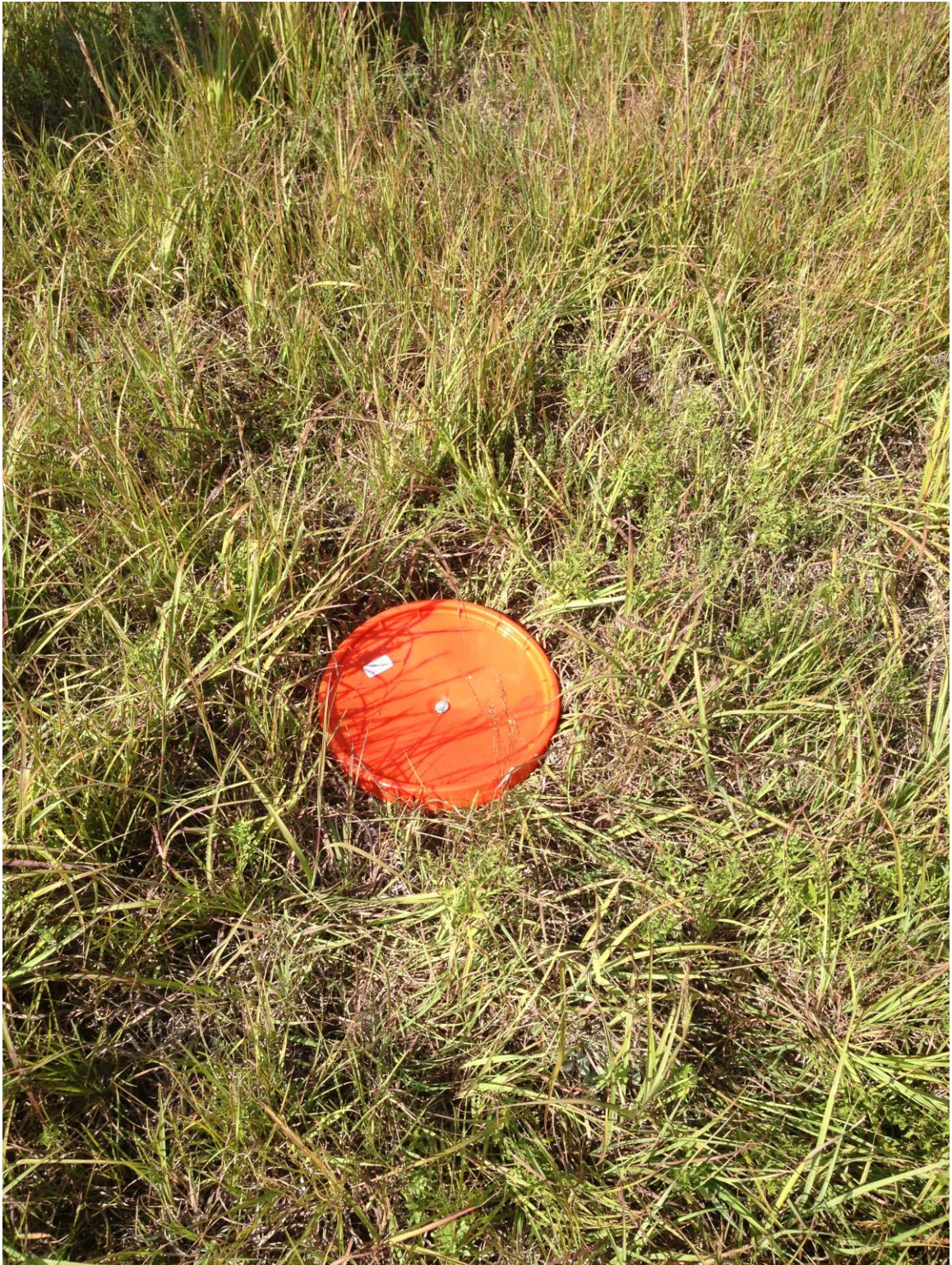
Figure 10: Image of one on-ground control points used in georectification of imagery.
