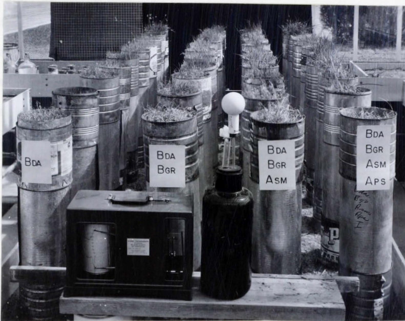
Figure 1. Buffalo grass (Bda) on left and sods containing buffalo grass, blue grama grass (Bgr), western wheatgrass (Asm), and western ragweed (Aps) on the right. Instruments are hygrothermograph (left) and atmometer apparatus. Series I (8 phytometers) is nearest camera.
