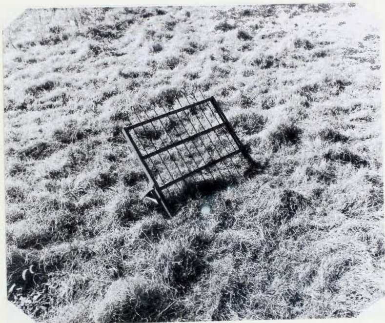
Fig. 2. Point contact apparatus used in analyzing vegetation within and surrounding each enclosure.
