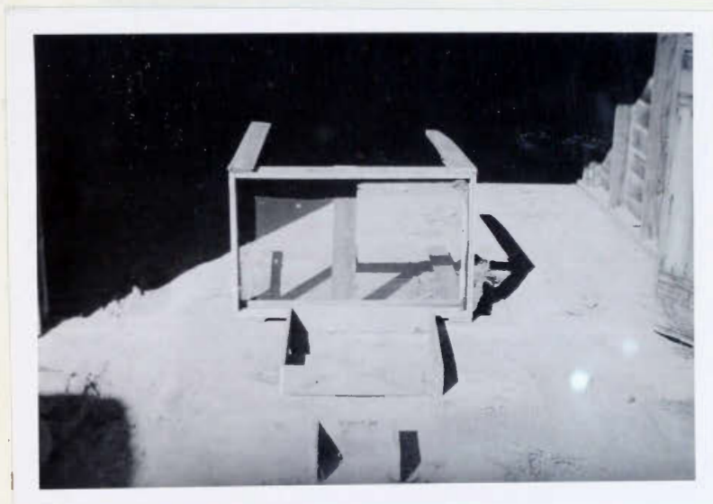
Figure 3. Equipment used in the removal of roots; an 8" by 8" form, a one-fourth square meter form, and a screen-bottomed washing rack.
