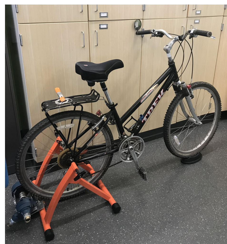
Figure 4: Bicycle powered water pump
