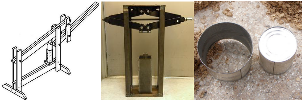
Figure 3: Press tools. (Left): Legacy Foundation briquette press. (Center) Car-jack based press. (Right) Can press.
