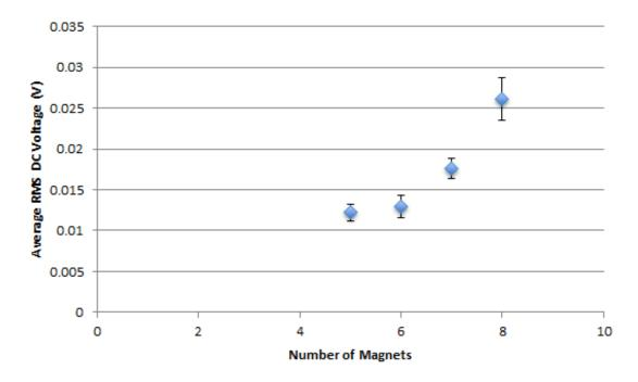
Figure 2. Effect of number of magnets on the average RMS voltage produced by the WEC device. The number of coils was 100 and the diameter of pipe was 1.27 inches. Error bars represent the standard deviation of triplicate measurements<sup>11</sup>.
