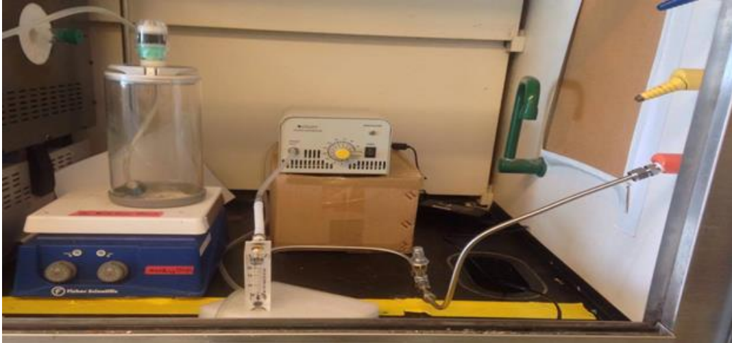
Figure 26. Laboratory-scale set-up of the ozonation system
