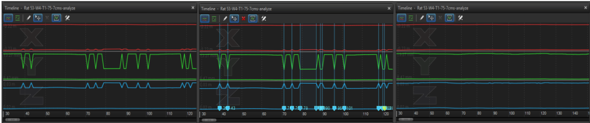
Figure 16. Stages involved to manually removing noise from a marker that is not moving. Note the noise spikes are all increased at the same magnitude and can easily be removed by selecting and moving them all. This noise profile was seen multiple times even when there was movement present.
