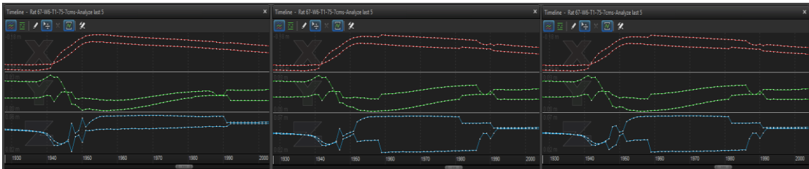
Figure 19. Examples of Noise Profiles and how they change from before being trajectorized (left), trajectorizing once (middle) and a second time (right). This tool helped in differentiating noise versus actual marker movement based on movement changes after trajectorizing.
