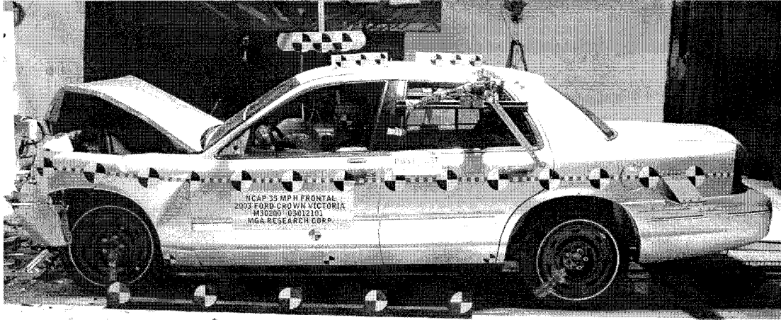
Figure 1. NCAP Test 4476 Ford Crown Victoria – Vehicle After Full-Frontal Barrier Test
