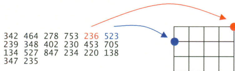
Figure 4-2: Mapping of 2D vGeo® data to configured grid.
