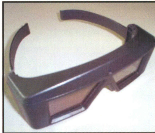
Figure 2-5: LCD shuttering glasses used for stereoscopic viewing.
