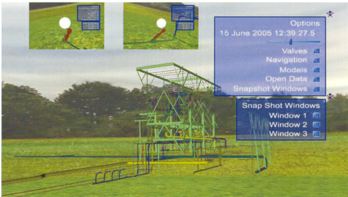
Figure 96: The option to save views and keep them at the top allows for the user to navigate away from objects and still oversee them.
