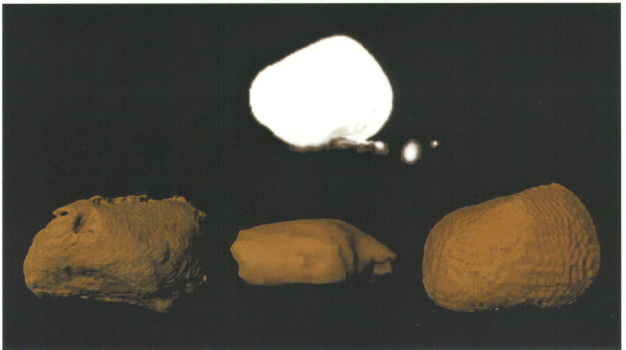
Figure 186: Michigan Dune sample from 5/31/05. On the far left is the X-ray reconstruction, followed by the old optical reconstruction algorithm and then the new reconstruction algorithm.
