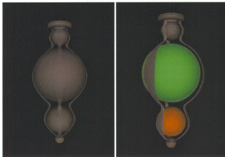
Figure 102: The visualization for valve state, with the top sphere corresponding to command, middle the state and the bottom the feedback.
