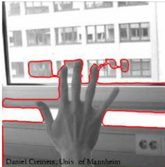
*Figure 3.* The active contour model fails to handle the topological changes of the moving fingers [13].
