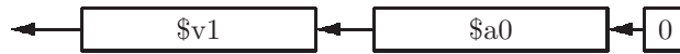
Figure 3.71: Diagram of a left shift on a pair of registers, $v1 and $a0
