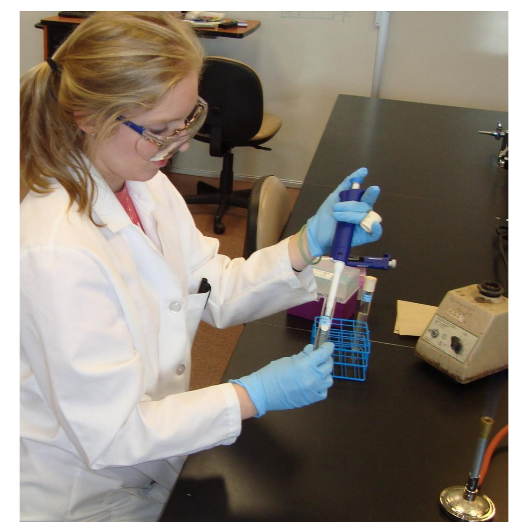
Figure 8. Creating the McFarland standard for the laboratory E. coli using a micropipette, vortex, and Bunsen Burner.
