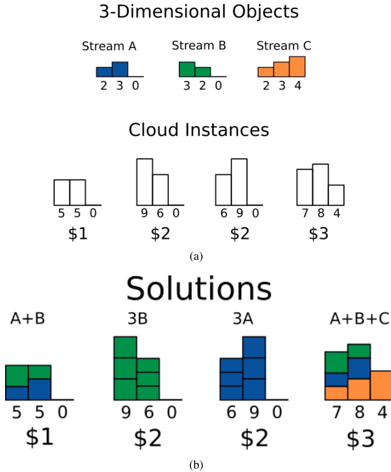
Fig. 2. (a) A three-dimensional multiple-choice packing problem. A - C represent three types of data streams whose resource requirements are expressed in three dimensions (CPU, Memory, and GPU). The heights represent the resource requirements, comparable to the width, height, and lengths of boxes. There are four choices of cloud instances each offering different sizes and costs. They are comparable to different types of trucks. The heights represent the sizes of these dimensions, comparable to the sizes of trucks. The goal is to fit the data streams (boxes) into the cloud instances (trucks). (b) Four possible solutions to accommodate different combinations of data streams.
