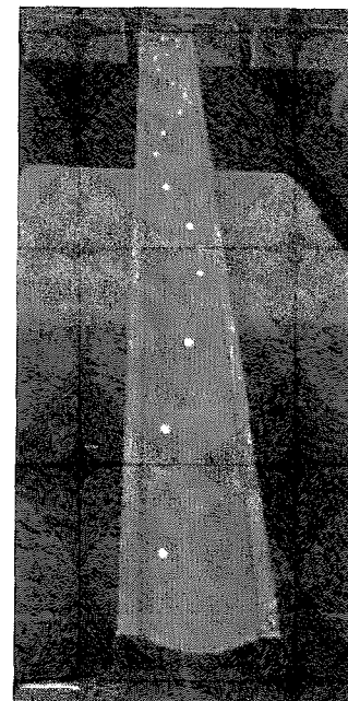
Figure 5.3: Combination of a linear motion on an inclined plane and a transverse oscillatory motion. Courtesy of Harvard Natural Sciences Lecture Demonstrations and Prof. Owen Gingerich. For more details, see http://sciencedemonstrations.fas.harvard.edu/presentations/scantling-and-ball .
