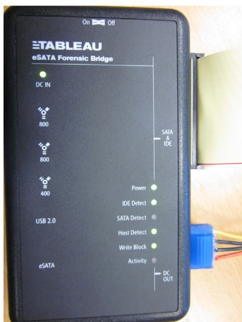
Fig. 1. Hardware write blocker.
