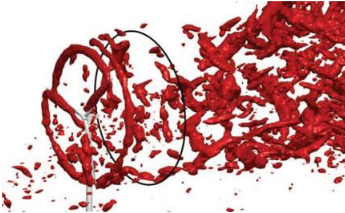
Fig. 6. Actuator line blade model with large eddy simulation (LES) wake model [30]
