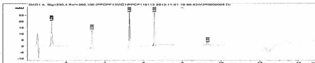
Figure 3: Chromatogram Ascentis 100mm x 2.1mm Column 0.5ppm Standard
