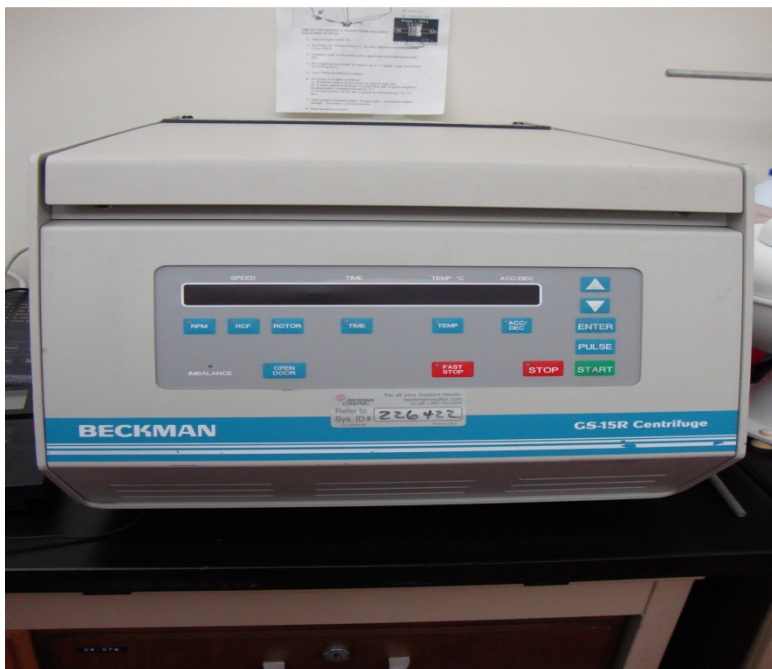
Figure-9: Centrifuge: Beckman CS-15R Centrifuge at 8898 RPM for 12 mins.
